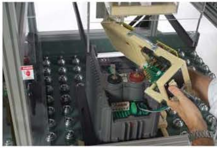
Adapter Palte to connect to UUT
