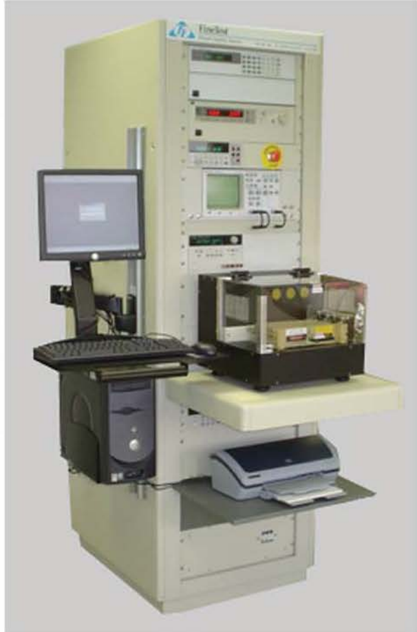
Test Fixture installed on ATE
