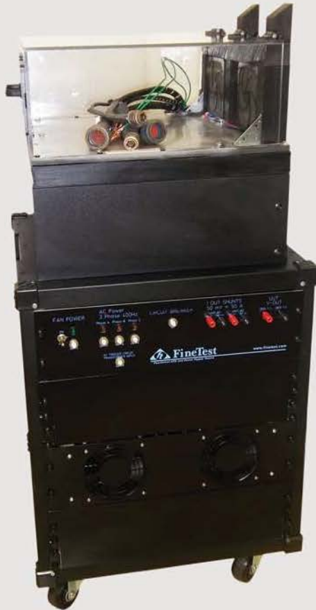
Front view Roll-Around ATP Fixture
