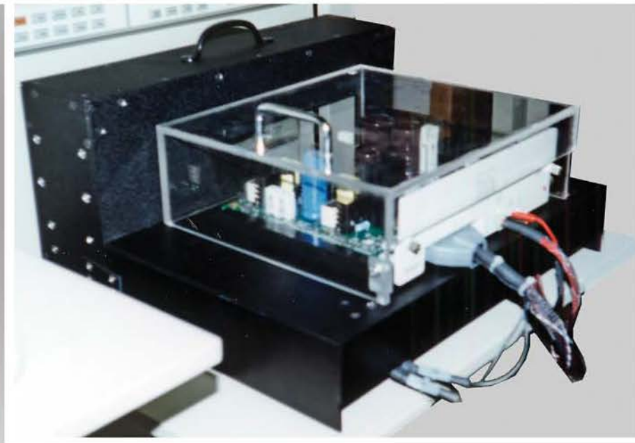
Side view of Test Fixture with a UUT
