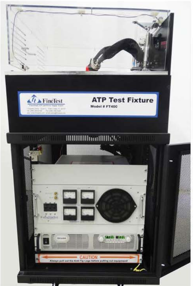
ATP Fixture with Safety Door Open
