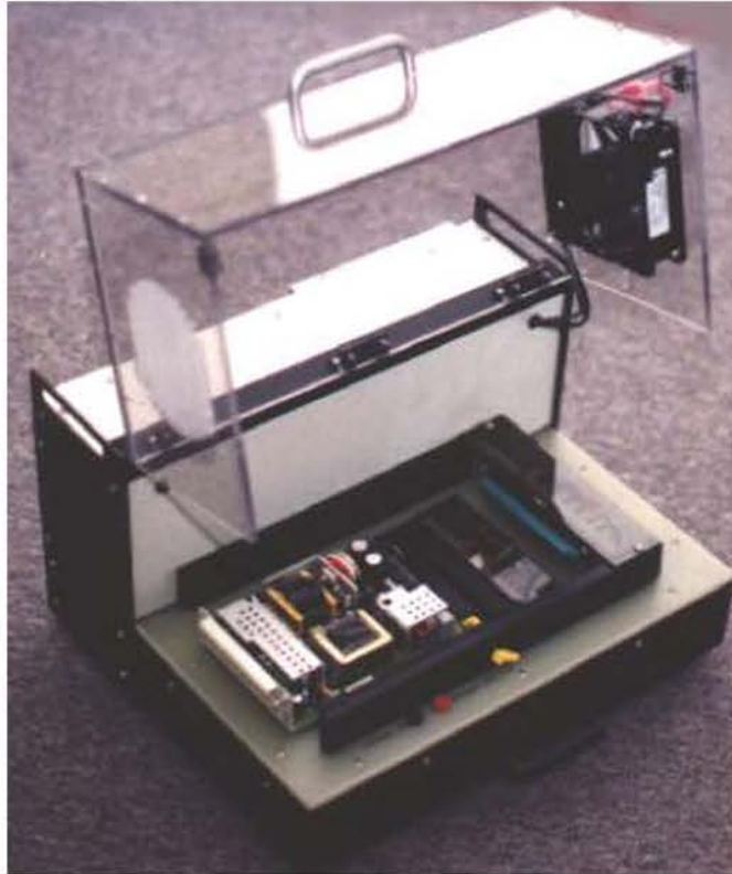
FineTest Test Fixture Kit with UUT
