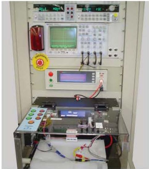
Test Fixture connected to HIPOT
