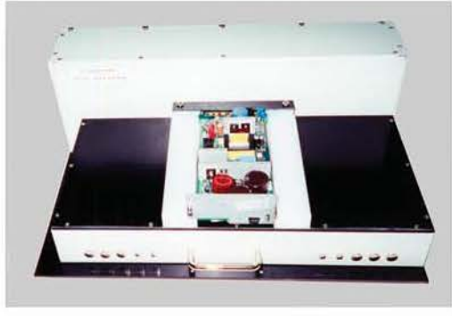
Power Module Test Fixture
