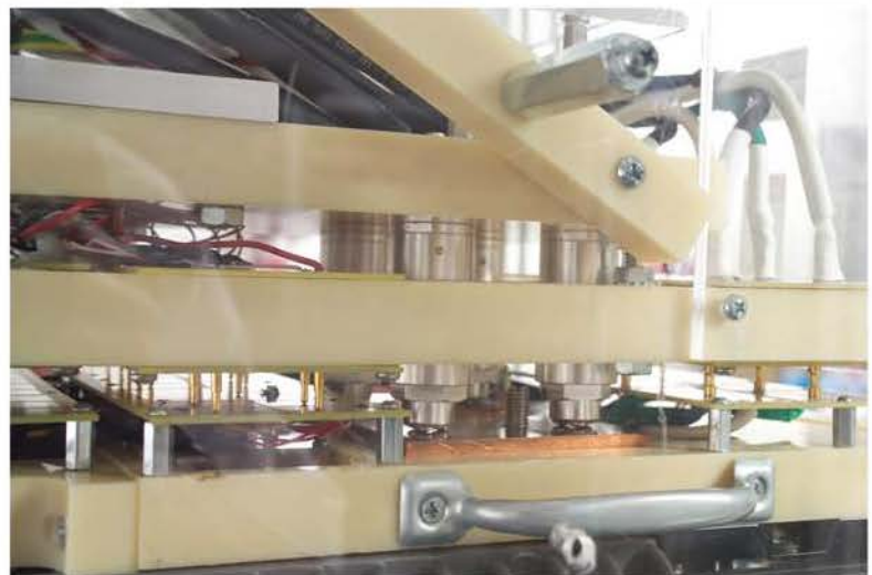
Close-Up of High Current Pogo-Pins
