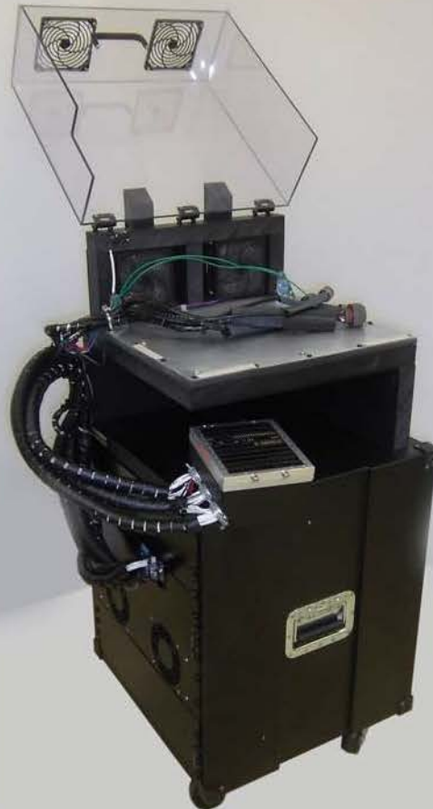
Rear view with Safety Cover Open showing Cable to Connect Fixture to ATE
