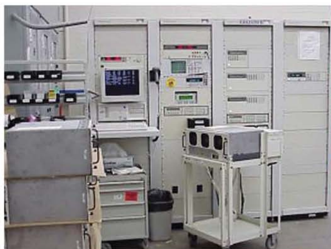
Cart and Cable Test Fixture with UUT
