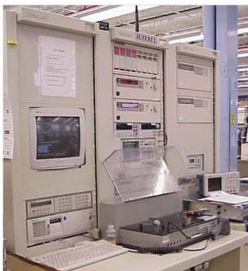
SMT Board Test Fixture
