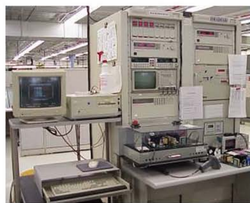
Test Fixture with UUT
