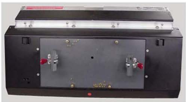
Front view Pogo-Pin Board Test Fixture
