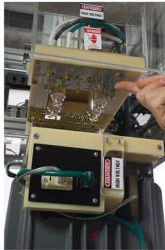
Fixture Top Pogo-Pins
