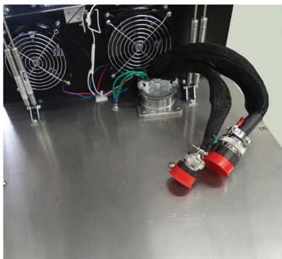
Close-up of the Fixture Top showing Mating Connectors, Gas Springs, and Top plate as a Heat-Sink
