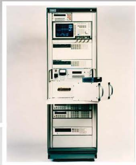
Plug-In UUT Test Fixture
