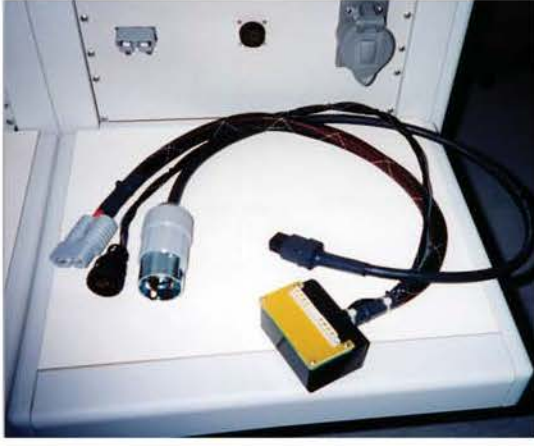
Cable to UUT Test Fixture
