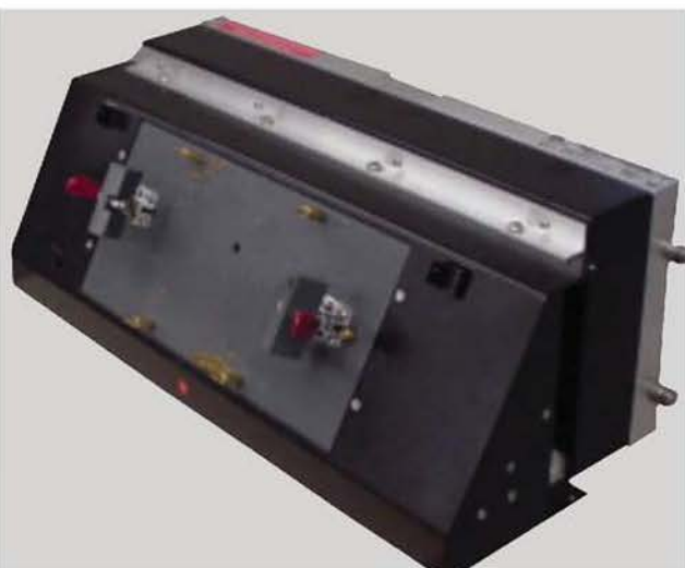
Side view Pogo-Pin Board Test Fixture
