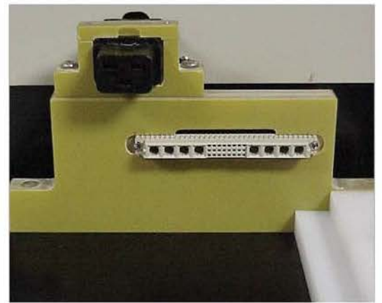
Close-Up of UUT Mating Connectors
