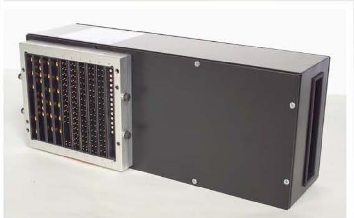
Fixture front with Virginia Panel Connectors
