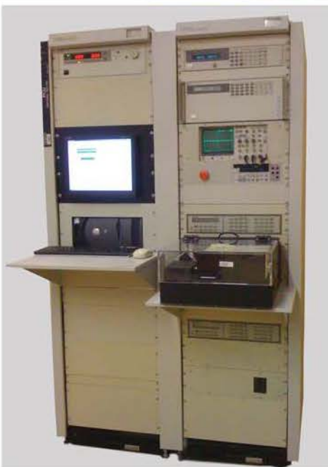
Tester with Test Fixture and UUT
