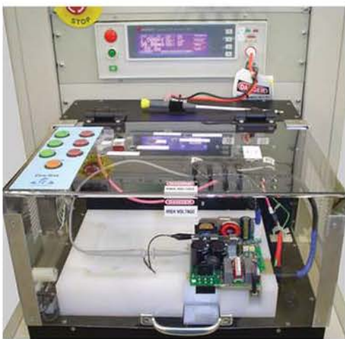
Close-Up Test Fixture with UUT
