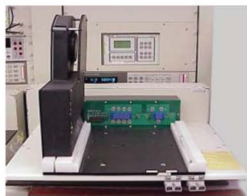
Fixture with PCB Mating Connectors
