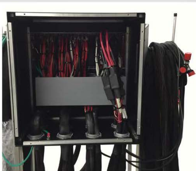
Inside ITA/Cable Harness wiring
