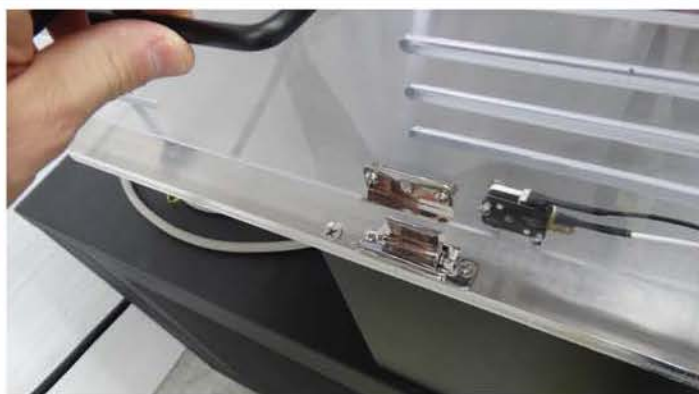
Safety Cover MicroSwitch and Latch
