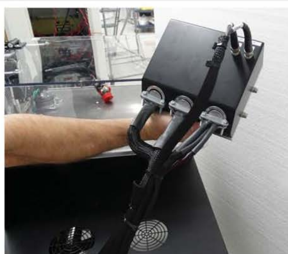
Cable to Connect Fixture to ATE
