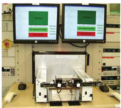
Dual UUT Test Fixture
