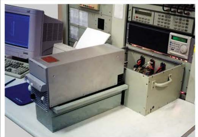
Plug-In UUT Test Fixture
