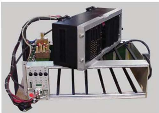
Card Cage Test Fixture
